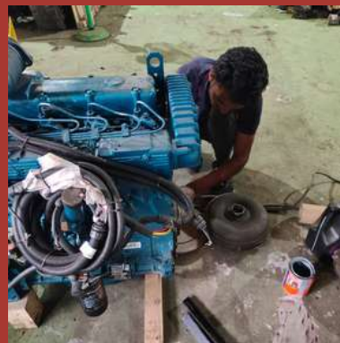
Modification and adoption of Kirloskar Engine in 7 T Hyster Forklift
